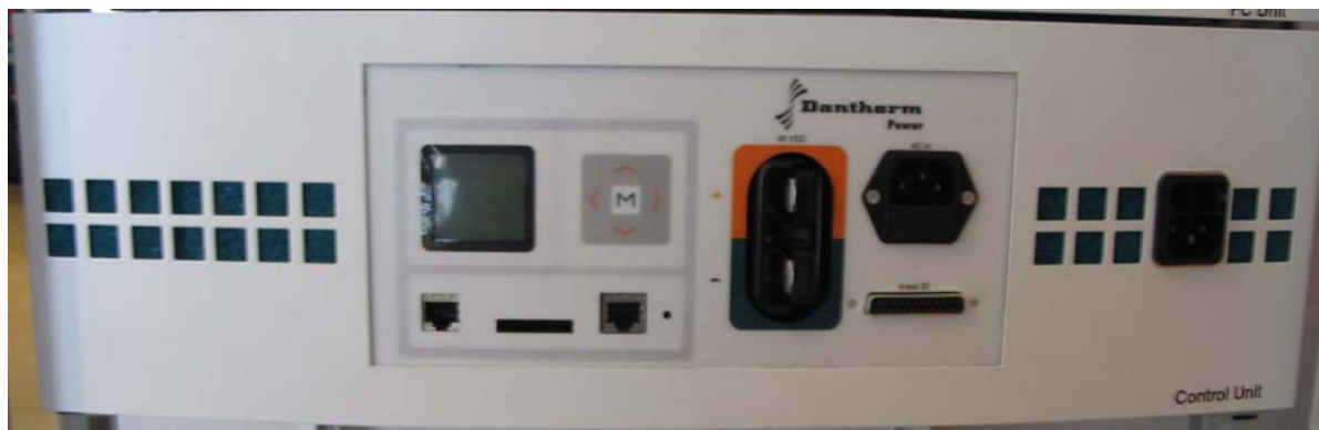
Front panel – Valve Block, Alarm, CAN, TCP/IP & LED's - AC-input, DC-out & current sharing
