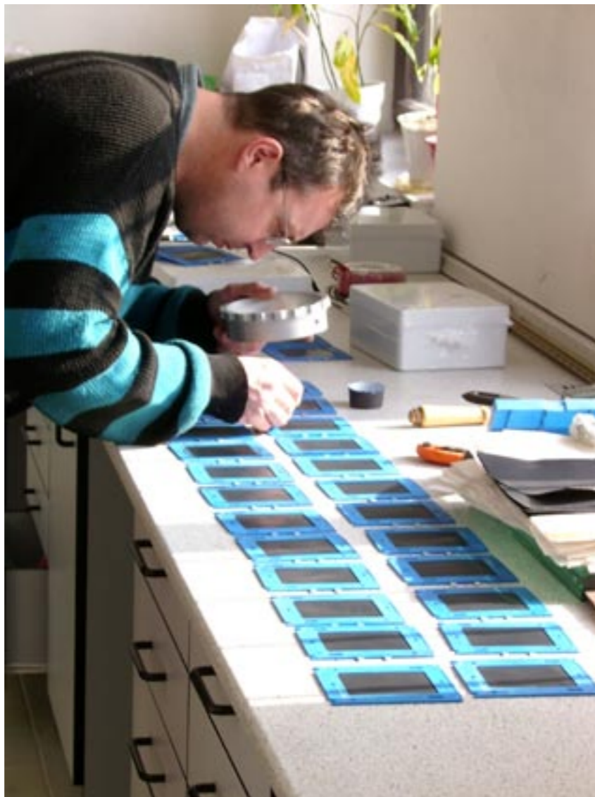
Visual check of the carbon plates
